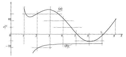
FIGURE 7. Second-order correction for the coefficient of local skin friction: (a) subcritical flow (F = 0.75); (b) supercritical flow (F = 1.5).
