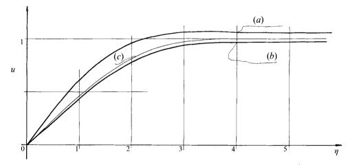
FIGURE 4. Total streamwise velocity in the boundary layer for x = 2.5,  $1/R^{\frac{1}{2}} = 0.006$ : (a) subcritical flow (F = 0.75); (b) supercritical flow (F = 1.5); (c) without the correction.
