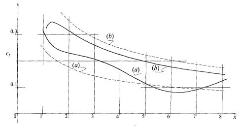
FIGURE 8. Coefficient of local skin friction for  $1/R^{\frac{1}{2}} = 0.0035$ : (a) subcritical flow (F = 0.75), (b) supercritical flow (F = 1.5); with the second-order correction (-----), without the correction (-----).
