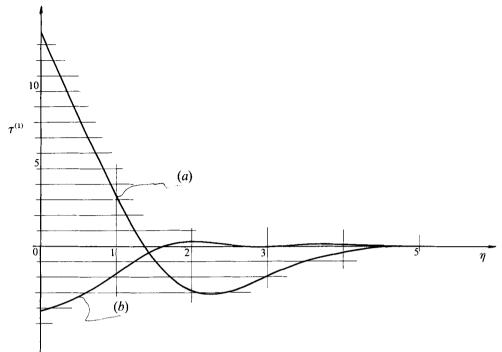
FIGURE 5. Second-order correction for the shear stress in the boundary layer for x = 2.5: (a) subcritical flow (F = 0.75); (b) supercritical flow (F = 1.5).
