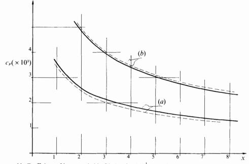
FIGURE 11. Coefficient of integrated skin friction for  $1/R^{\frac{1}{2}} = 0.0035$ : (a) subcritical flow (F = 0.75), (b) supercritical flow (F = 1.5); with the second-order correction (----), without the correction (-----).
