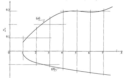
FIGURE. 13. Coefficient of local lift for  $1/R^{\frac{1}{2}} = 0.006$ : (a) subcritical flow (F = 0.75); (b) supercritical flow (F = 1.5).
